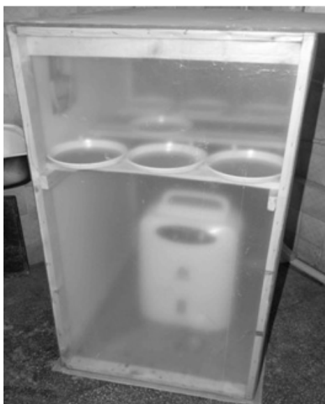
Phot.: Honey dehydrator box – front view.
