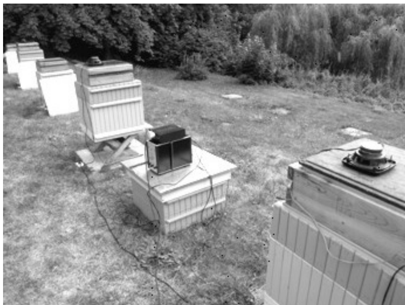
Photo 1. A set of equipment used for venom collection using combined electrical and sound
